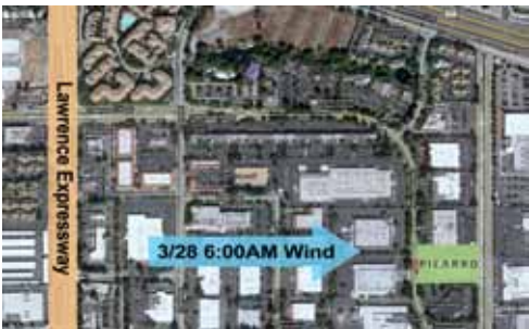
Fig 2: Ambient air measurements were made by a Picarro G2401 from the Picarro roof sampling line (Picarro location shown to right as 'A'). The CO and CO 2 concentration data is shown below show spikes during commuting hours. Wind direction during that time period was West, bringing in air
