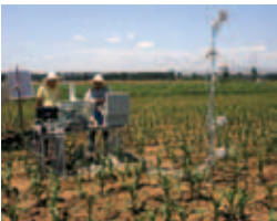
Sampling tower, Picarro (left) and cryogenic trap (right). Lowest-level sample inlet at ground level (lower right).
