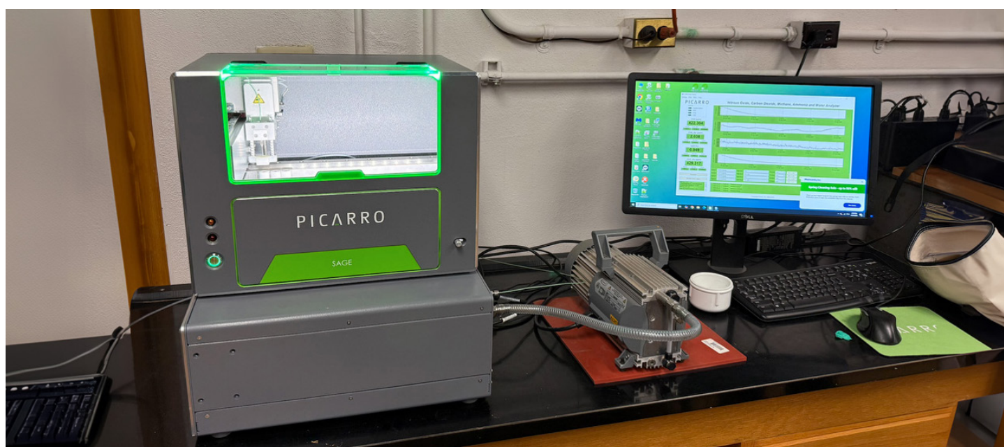
Figure 1. The setup of the Sage gas autosampler and G2508 analyzer at UC Berkeley.
