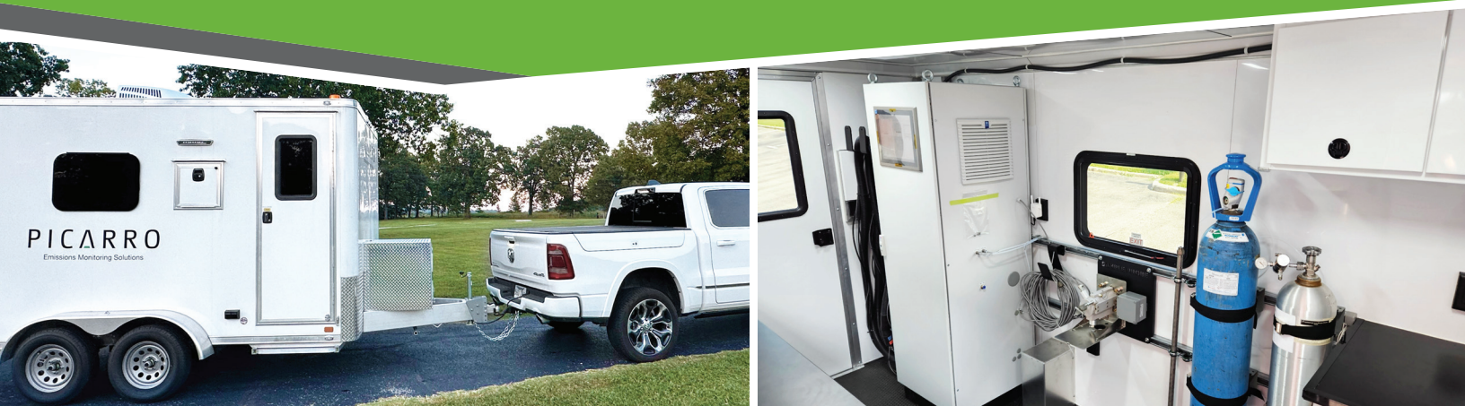
Figure 1. The Picarro CEMS shown here is our demonstration platform designed to meet all current and upcoming performance requirements and regulations for EtO monitoring, including PS-19, OTM-47, and others.
