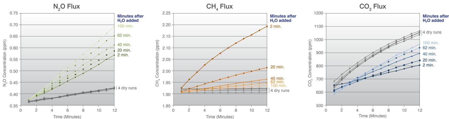
**Simulated rain event in closed-system chamber lab study:** Concentration time series for dry and wet dirt measurements of N<sub>2</sub>O, CH<sub>4</sub> and CO<sub>2</sub> are shown. After adding water, N<sub>2</sub>O emission rate triples in 2 min and continues to rise, while CH<sub>4</sub> emission rate spikes and then decreases, and CO<sub>2</sub> emission rate is suppressed but recovers slowly. Contact Picarro for more details and the latest data related to this study.
