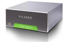
Excellent measurements of  $CH_4$  are only possible if the influences of other molecules in the sample are quantified. The G2132-i makes precise measurements of  $CO_2$  and  $H_2O$  concentrations to allow the cross-influence of these species to be quantified and corrected while providing more insight into the sample. The analyzer comes equipped with ChemDetect<sup>TM</sup>, a new layer of analysis that inspects the recorded spectra to find indications of contaminating species.
