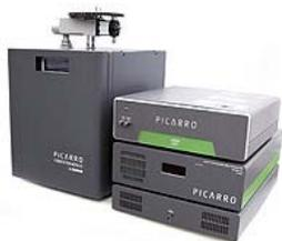
Combustion Module-CRDS for  $\delta^{13}\text{C}$  analysis of imported honey and detection of adulteration.
