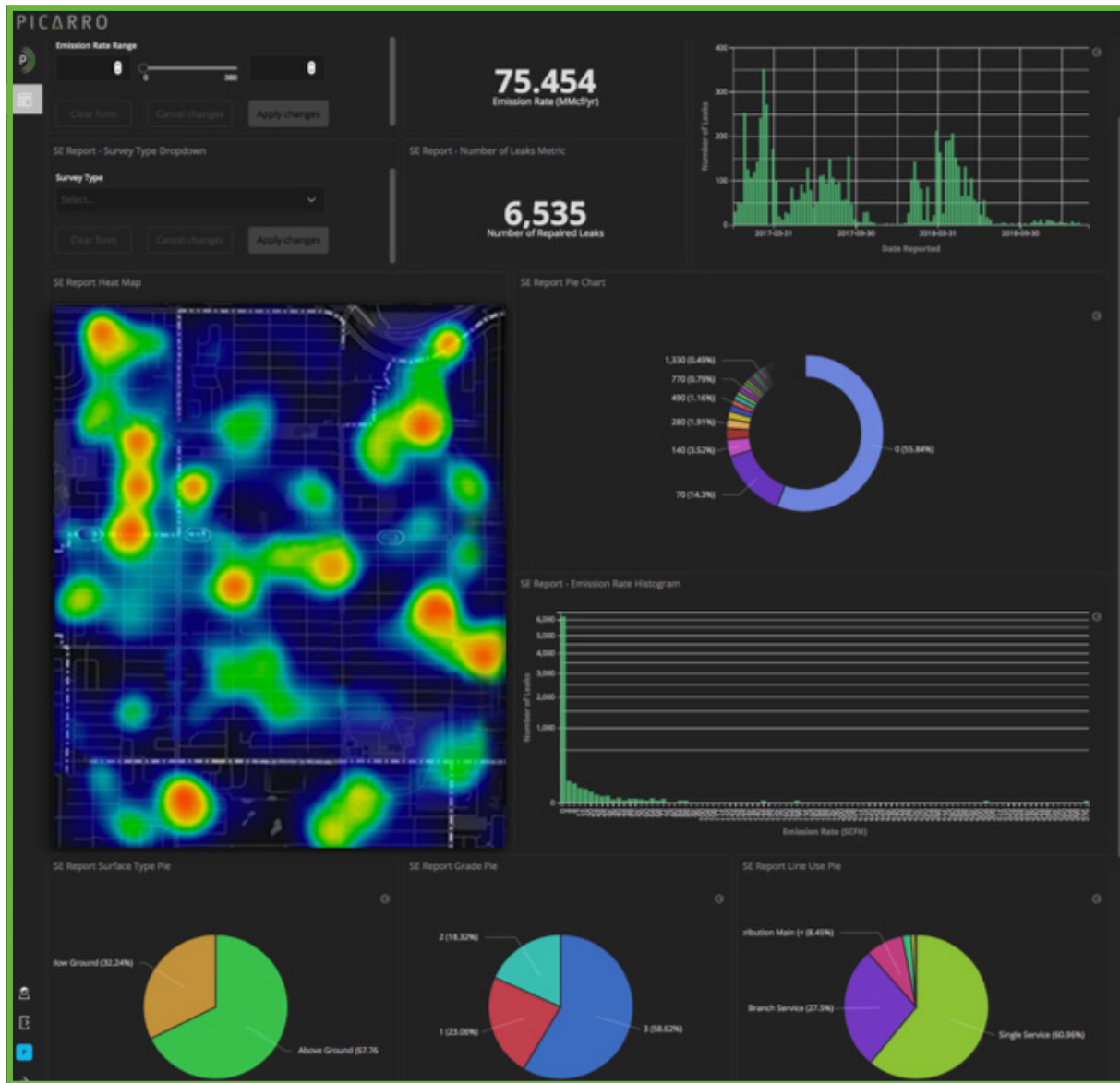
Figure 1. Picarro's Emissions Quantification Analytics dashboard used for super emitter leak identification and analysis. The dashboard allows gas operators to quickly look at repair scenarios, calculating aggregate emissions reduction benefits of different types, sizes and locations of leaks.
