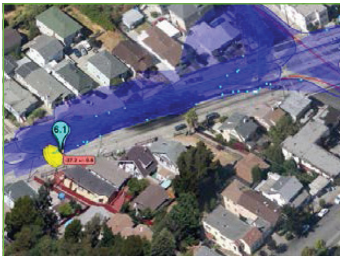
Figure 3. Picarro leak indications and leak location.
