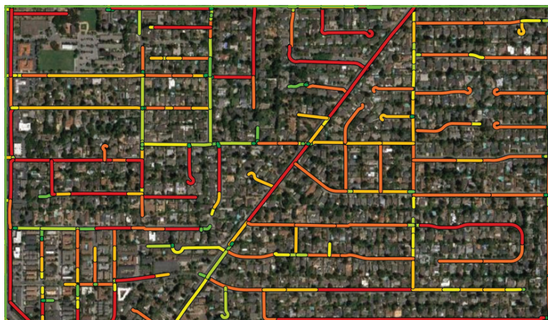
Figure 1. Leveraging methane data to prioritize pipe replacement at the project level earthquake to do a rapid, post-disaster survey of Napa's entire gas infrastructure.
