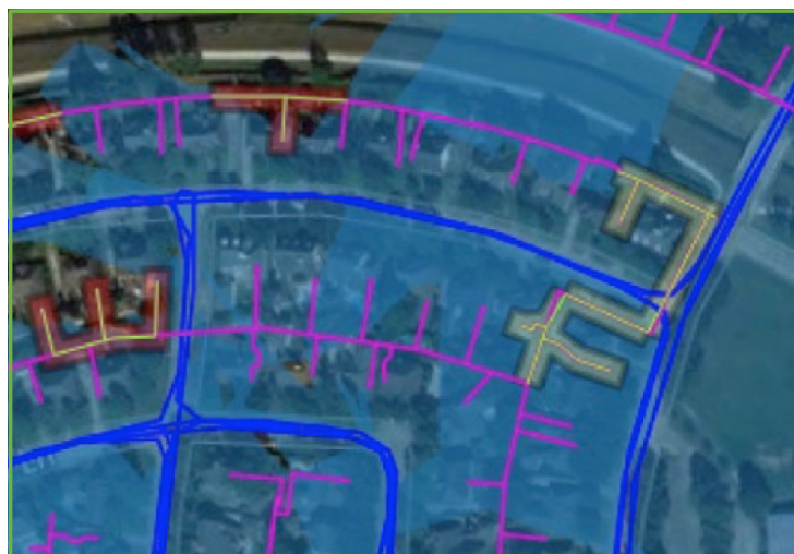
Figure 2. Example of compliance survey report output showing blue vehicle breadcrumb, magenta GIS assets (gas mains/services), blue shaded FOV coverage area, and assets associated with a leak indication highlighted in yellow and assets associated with a gap in FOV coverage highlighted in red.
