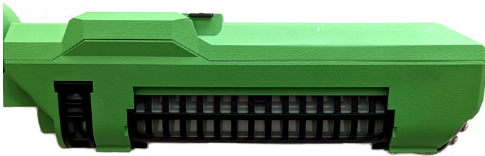
Figure 1 The unit uses diffusion sampling and an OPLS sensor.
