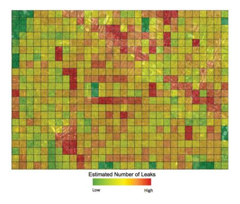
Figure 2. Below-ground leak density within grids as estimated by Picarro methane measurements and associated analytics. Desirable grid sizes often vary from a few city blocks to a square mile for example). Grids with high predicted leak density are prioritized for more frequent leak survey and those with low predicted leak numbers are surveyed less frequently. Methane data is collected across the entire infrastructure approximately every year to enable this analysis.
