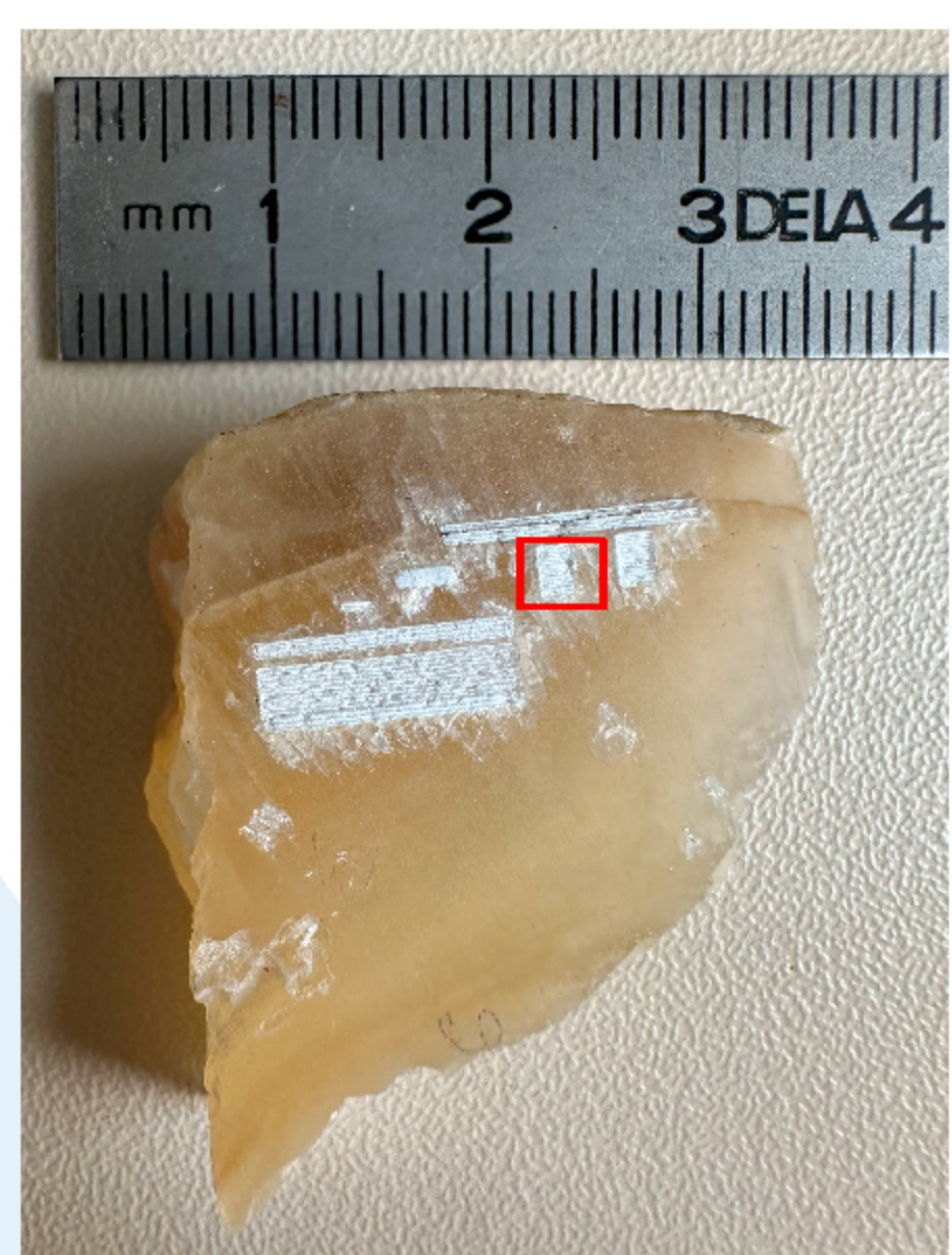
Figure 6. V11 Stalagmite (Bihor Mts., Romania) fragment used for the preliminary testing. Ablated area highlighted by the red rectangle.
