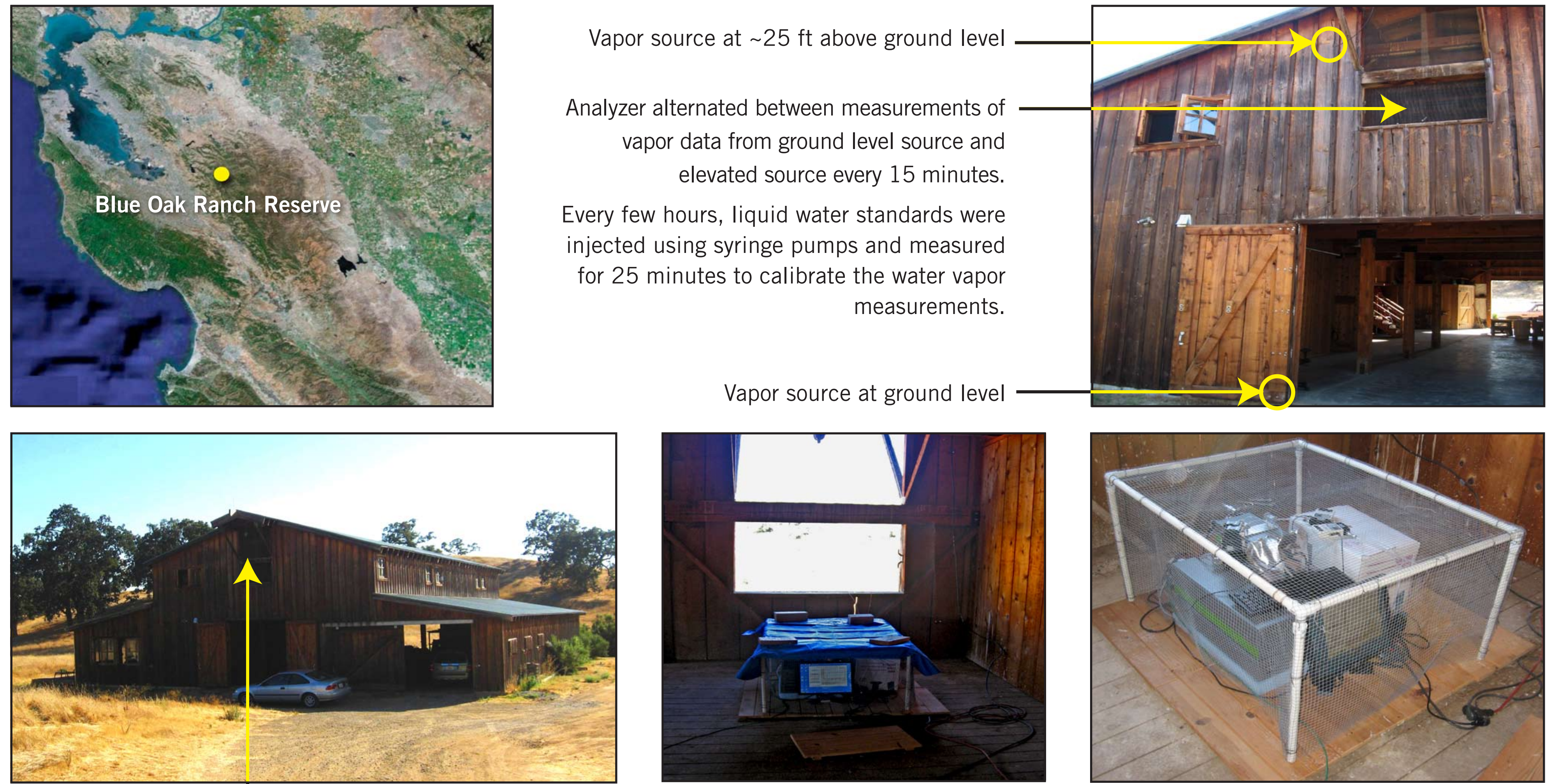
Field-deployable Picarro Isotopic water vapor analyzer with robust automated liquid calibration module installed on the top floor of the barn
