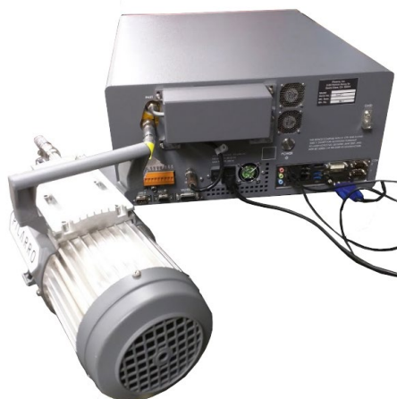
Figure 13: Analyzer and Pump Connections
