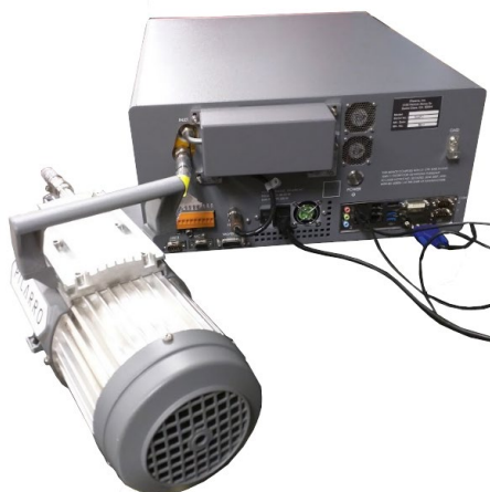
Figure 7: Analyzer and Pump Connections
