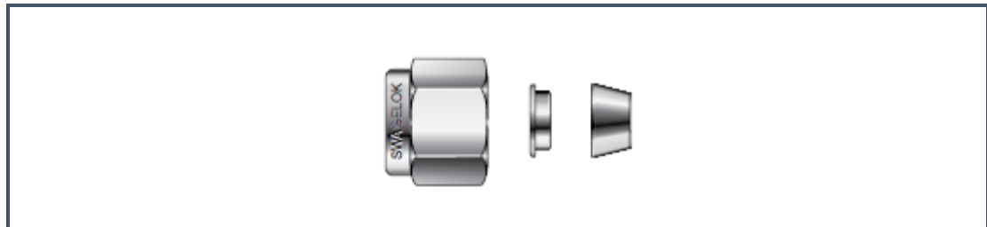
Figure 7: Orientation of ferrules and nut
