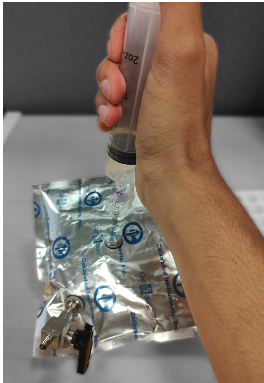
Figure 35 - Filling a syringe from a gas bag
