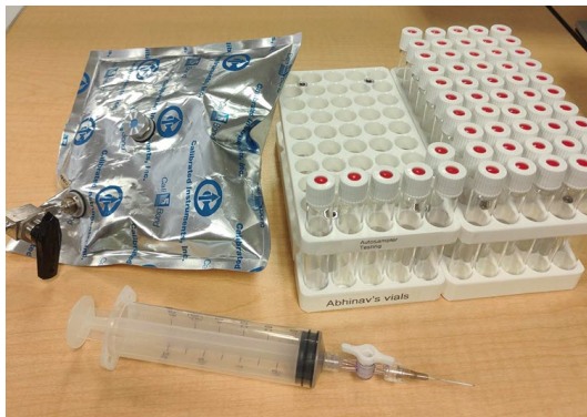
Figure 34 - Preparing to fill vials from a gas bag
