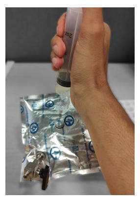
Figure 27 - Filling a syringe from a gas bag
