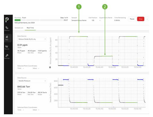
1 Vial data with good needle pressure 2 Vial data with poor needle pressure
