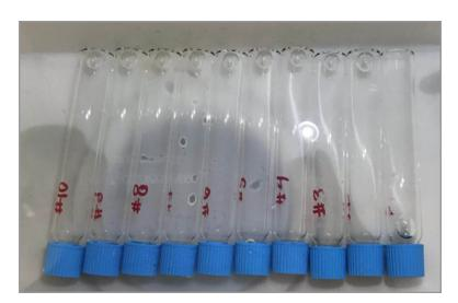
Figure 35 - Vials filled with water, showing equal small bubbles, indicating good vials
