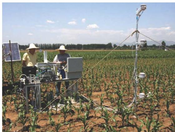
The isotope analyses can allow the partitioning of evapotranspiration into its components: soil evaporation and leaf transpiration. Once daily, during the vapor measurements, liquid water isotope standards were measured by the Picarro analyzer using its included autosampler and subsequently used to calibrate the vapor-phase data.
