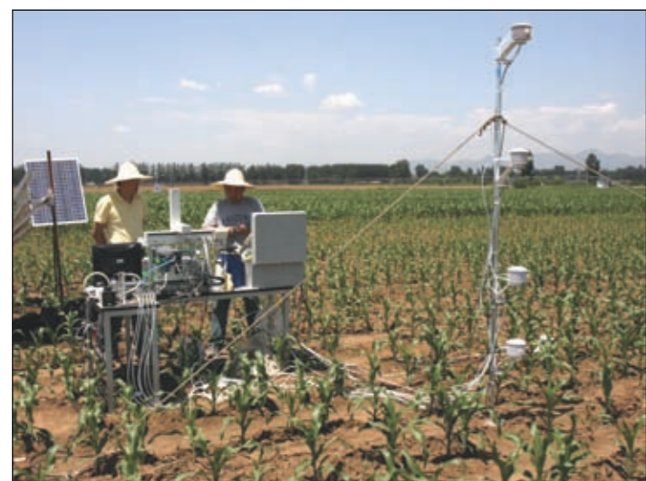
Sampling tower, Picarro (left) and cryogenic trap (right). Lowest-level sample inlet at ground level (lower right).
