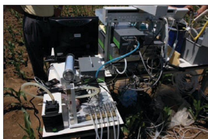
Picarro analyzer, sampling manifold, pump and rotary valve
