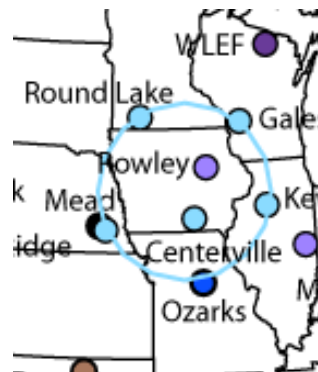
Figure 7. The Penn State Ring 2 project is using WS-CRDS instrumentation and other technologies to measure the entire CO 2 flux of a region roughly spanning the state of Iowa.
